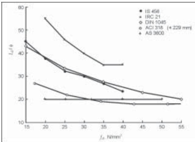
Fig 2 Comparison of  $L_d / \phi$  values for compression bars<sup>3</sup>
