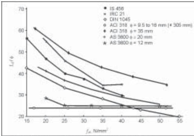
Fig 1 Comparison of  $L_d / \phi$  values for tension bars<sup>3</sup>
